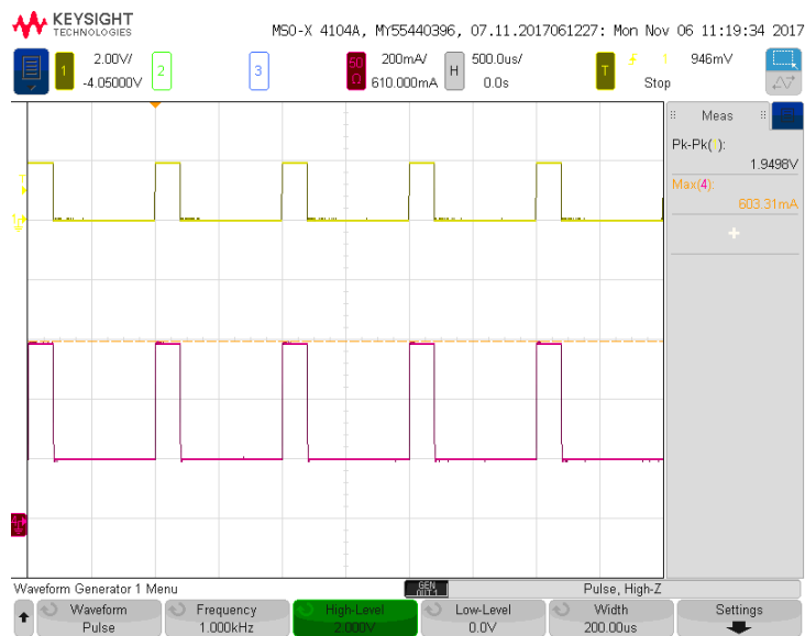
Fig. 10: Pulsed operation with offset; yellow/upper trace: Input voltage CA-DCSP; red/lower trace: Output current
