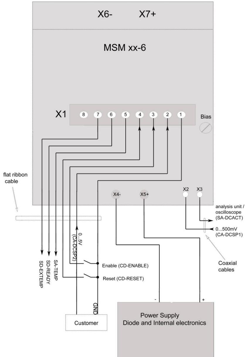
Wiring Diagram for MSM xx-25 and MSM xx-50
