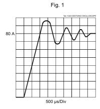
Diode current at a set point step function from 0 to 80 A.
