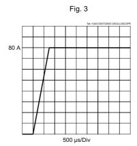
Diode current at a set point step function from 0 to 80 A.
