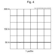
Diode current at the alloying of an individual diode in the stack.
